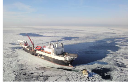
Figure 6 - Pipelaying in the Gulf of Finland (Source: Allseas)
